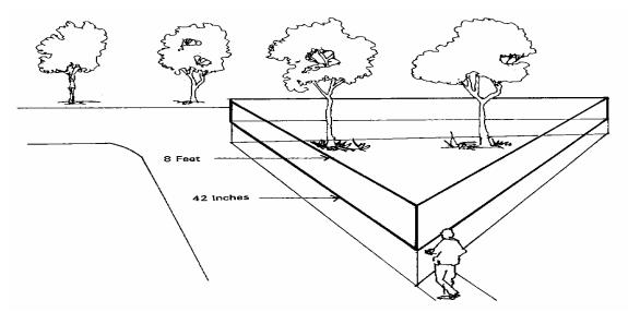
NOTE: The area of a sight distance triangle between 42 inches and eight feet above the existing street grade shall remain open.
