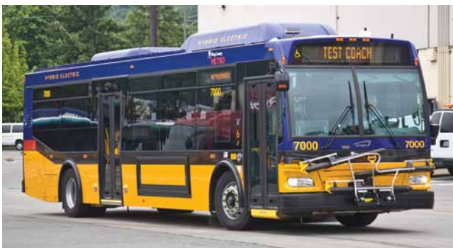
New forty-foot, low-floor Daimler/Orion hybrid buses can get up to 5.7mpg
