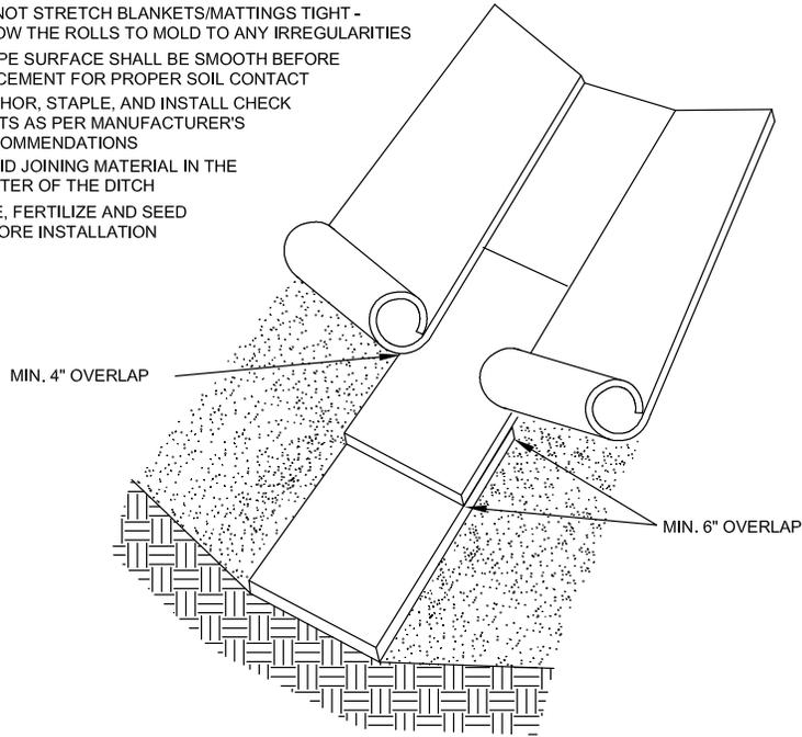
**FIGURE C.3.3.B SLOPE INSTALLATION**
