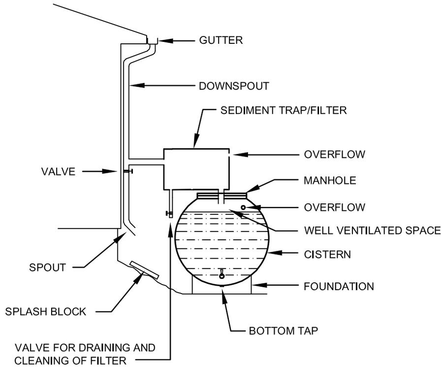
**FIGURE C.2.7.B VARIOUS POSSIBLE RESERVOIR CONFIGURATIONS (STENSROD, 1978)**
