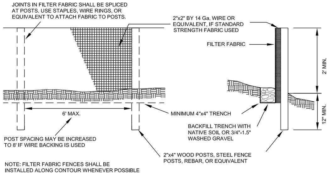
**FIGURE C.3.6.B SILT FENCE INSTALLATION AND MAINTENANCE**
