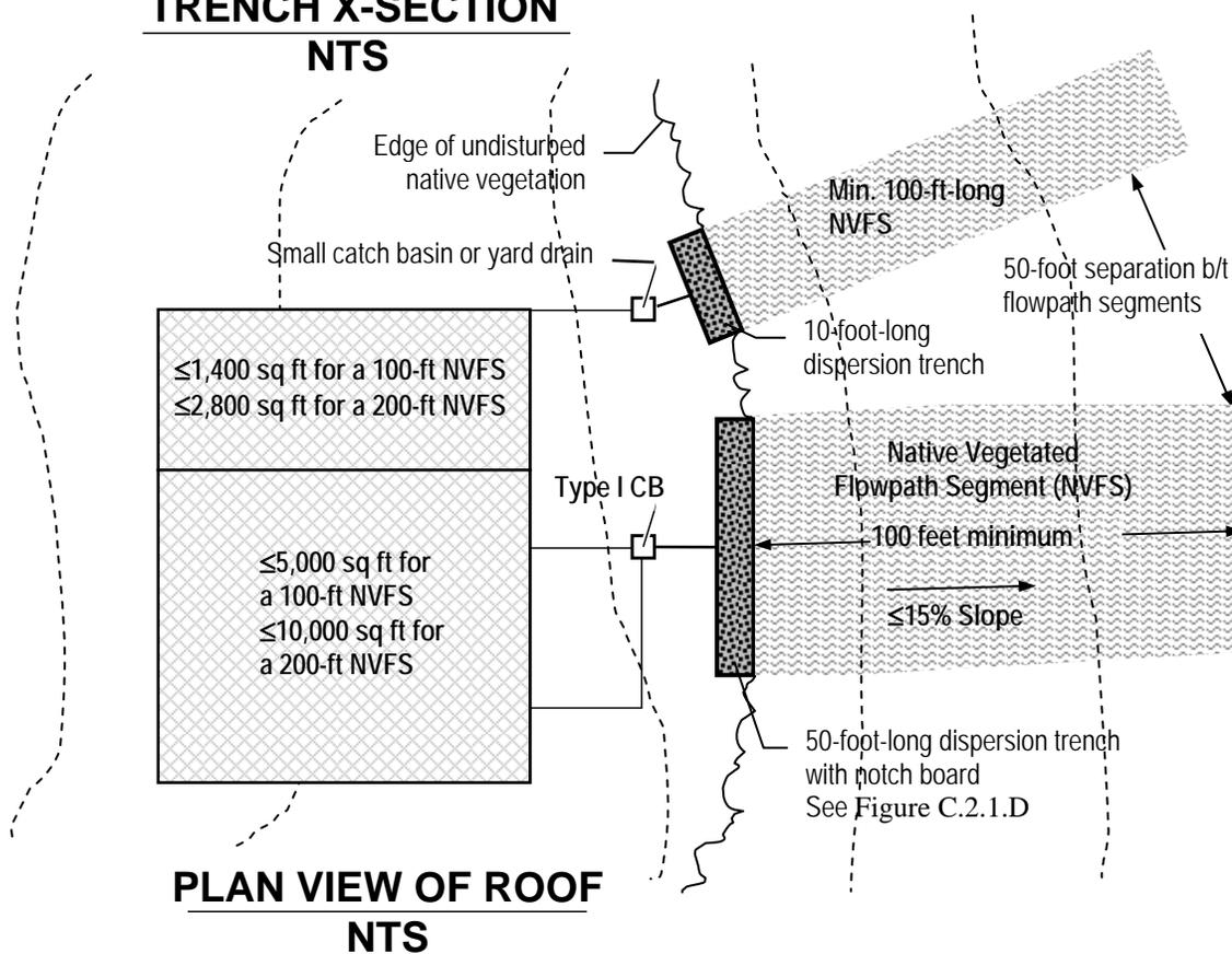
**FIGURE C.2.1.D 50-FOOT DISPERSION TRENCH WITH NOTCHED BOARD**
